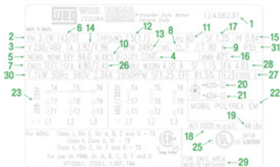
Figure 17 - Nameplate layout for frames 143T to 215T
